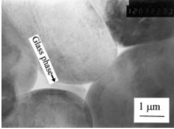
Fig. 4. TEM microstructure of Y-TZP/LAS-glass with the glass content of 2 vol%.
